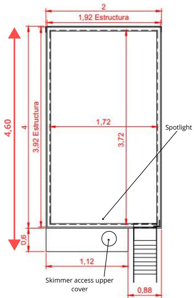
**Mobile ladder.** It can be positioned on either side of the pool.
